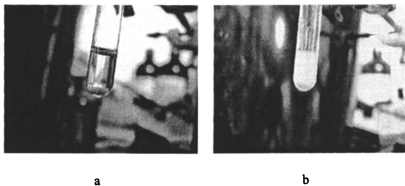
Figure 4 An aqueous solution of polymer 2, at room temperature (a) and after heating (b)
